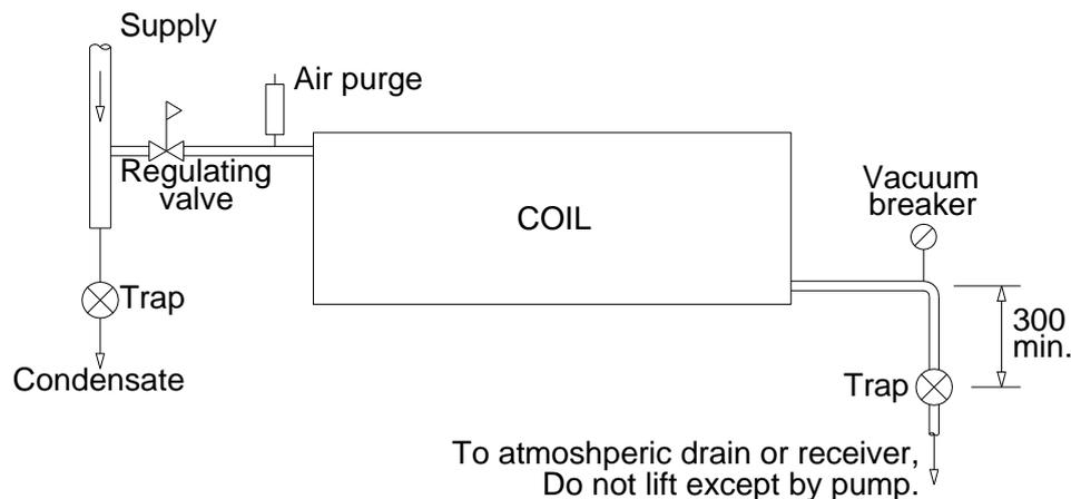
The steam trap should be 1 to 3ft (0.3 to 0.9m) below the bottom of the steam coil to provide a hydraulic head of approximately 0.5 to 1.5 psig (3.5 to 10.3kpa above atm.). Location of the trap at less than 12in (300mm) minimum usually results in improper drainage and operating difficulties.
